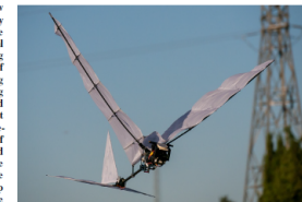
Figure 1. Front view of the flying E-Flap robot during a downstroke.
